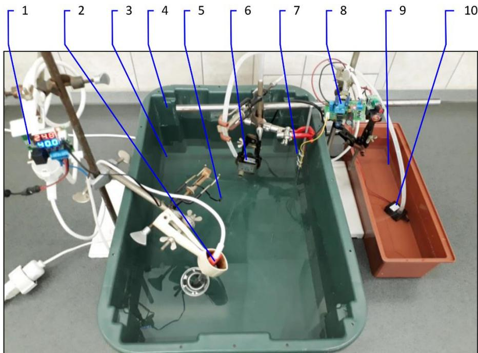
*Figure 1. The temperature-regulated water bath system (1 – W1209 digital thermostat; 2 – immersion heater; 3 – water bath; 4 – PP harvest crate; 5 – NTC waterproof temperature sensor; 6 – aquarium pump; 7 – liquid level sensor; 8 – liquid level controller; 9 – replenisher for the water bath; 10 – submersible water pump)*
