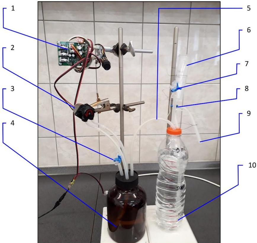
*Figure 2. The anaerobic digester system equipped with mixer (1 – motor speed controller; 2 – 12V DC motor with peristaltic pump; 3 – flushing tube with stopcock; 4 – reactor; 5 – tube for biogas departure; 6 – a barrel of a 50 ml syringe to refill the confining liquid container; 7 – flushing tube with a stopcock; 8 – directional control valve; 9 – confining liquid overflow; 10 – confining liquid container)*
