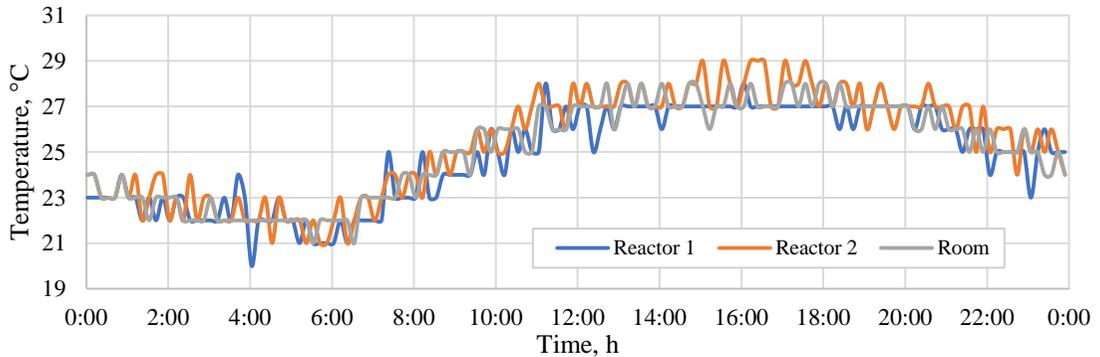
Figure 5. The temperature of the room and the inner temperature of the two room-temperature reactors
