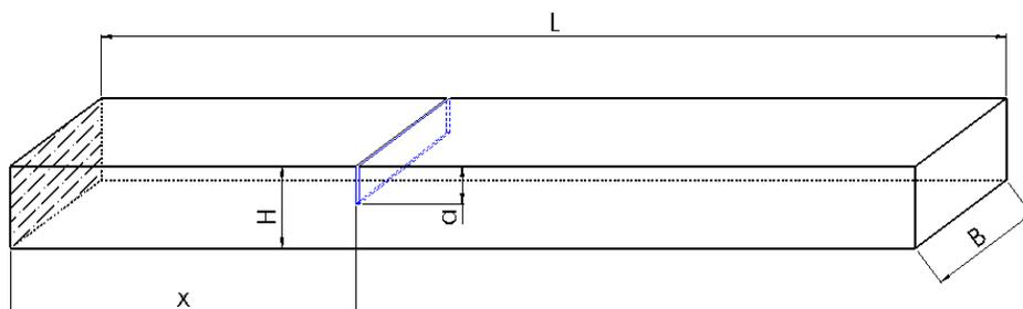
*Figure 1. Main dimensions of the cantilever beam*
