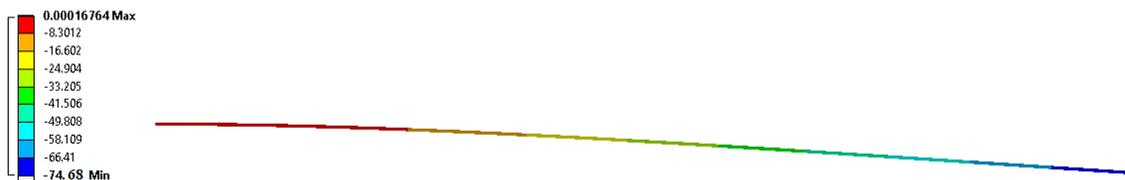
Figure 2. Deflection under own weight for the 1200x20x4 mm cantilever in
