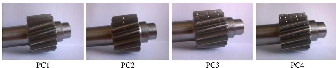
Figure 2. Pinions with different failure status
