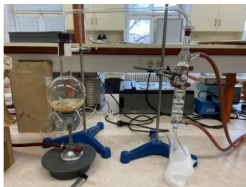
Figure 3. Testing the measurement of alcohol content
