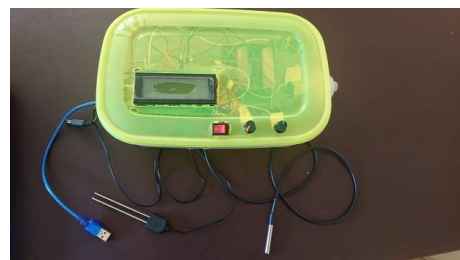
Figure 8: Final prototype of the irrigation control device before assembly. Figure 9: Final prototype of the irrigation control device
