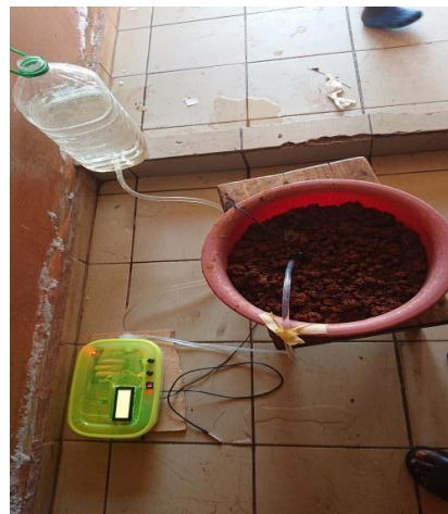
Figure 12: Installation of the device for humidity monitoring
