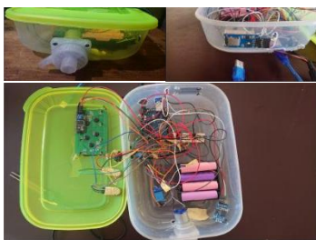
Figure 8: Final prototype of the irrigation control device before assembly. Figure 9: Final prototype of the irrigation control device
