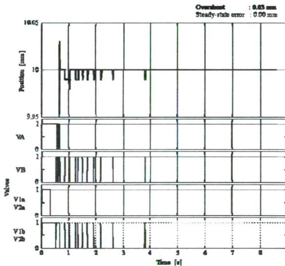
**Fig. 4. The time functions of the position and control signal**
