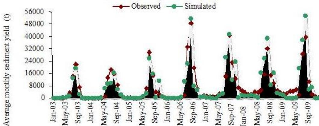
Fig. 8 Observed and simulated sediment flow for calibration period (2003–2009)
