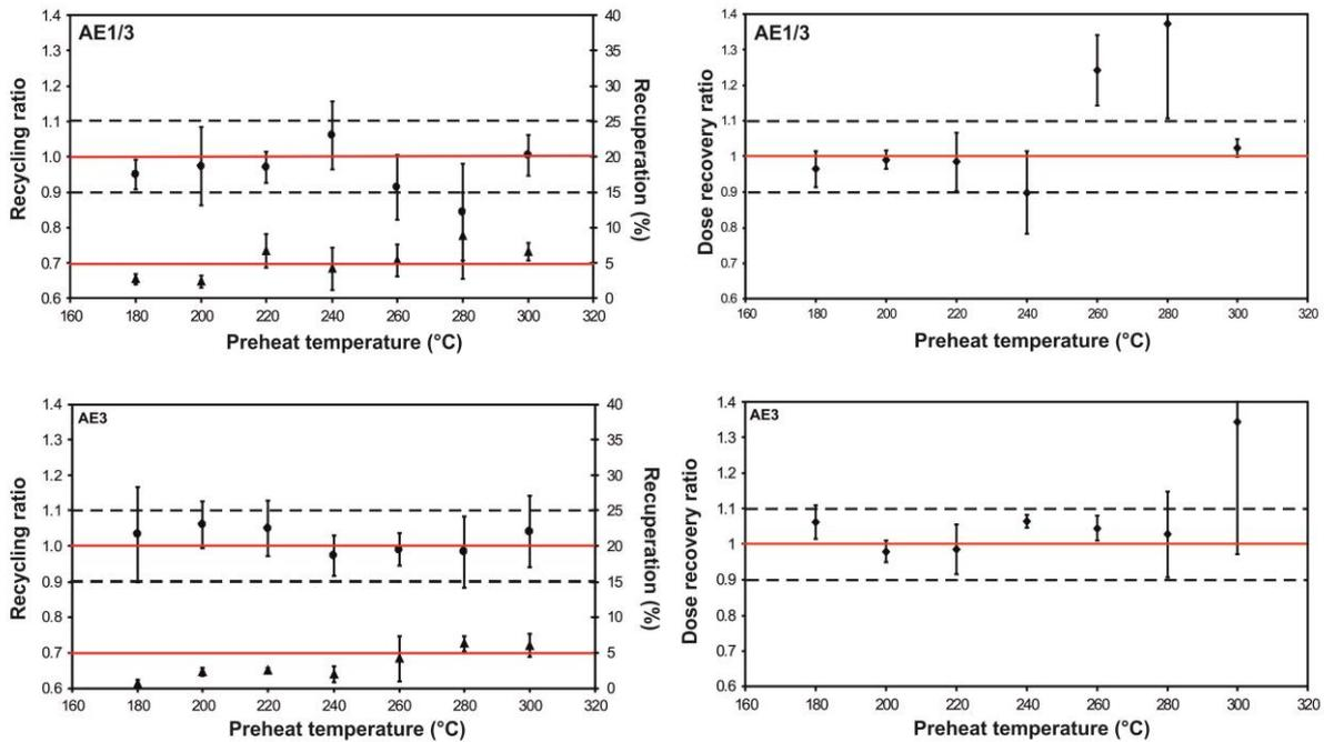
Fig. 3 Preheat and dose recovery tests of the samples. The red line and the dashed line mark the three criteria and the errors of the criteria
