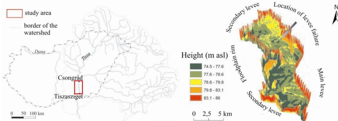
Fig. 1 The study area is located on the Lower Tisza. In the model the flood would destroy the levee and inundate a flood protected area (reservoir)
