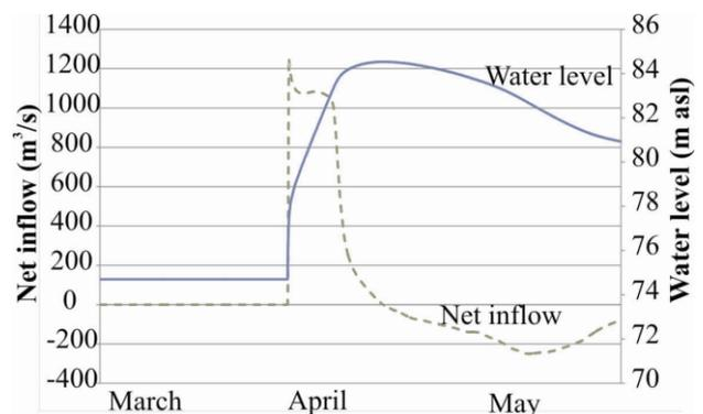
Fig 2 The water level and the water inflow curves of the reservoir in the case when the levee breached before the peak-flood at 958 cm stage
